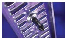
Grates are supplied with a 'QuickLok' locking stud which push fits into a stainless steel spring clip in the 'QuickLok' locking bar. To remove grate, put removal hook into grate opening and pull upwards. Heel guard stainless steel Class A
